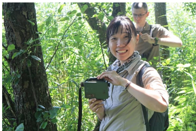
An autonomous recording unit (ARU), which can be programmed to record on a predefined schedule (e.g., time of day). Photo by Gintas Janulis.
